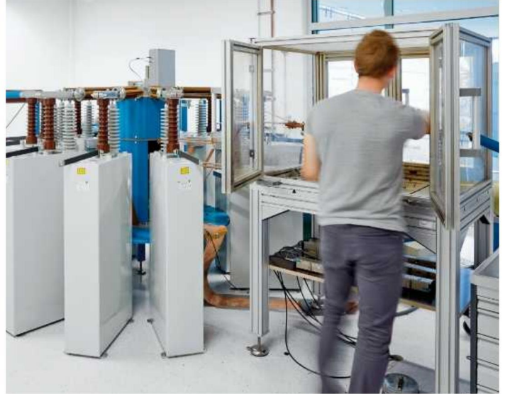
Fig. 27: Lightning surge current generator
